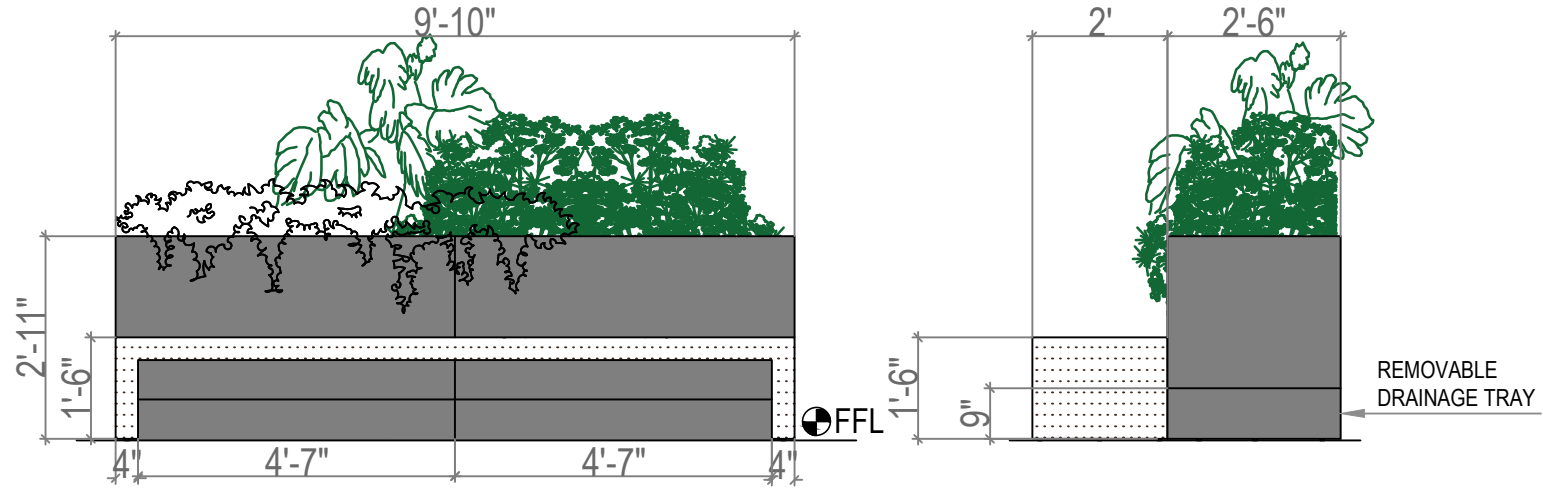
1.1 PLANTER WITH INTEGRATED SEATING - ELEVATION GROUND FLOOR
