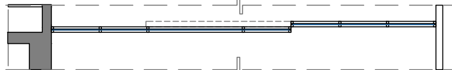
3.3 - 3.4 MS FRAMED GLAZED PARTITION AND MS FRAMED SLIDING GLASS DOOR - PLAN FIRST FLOOR - FOYER
